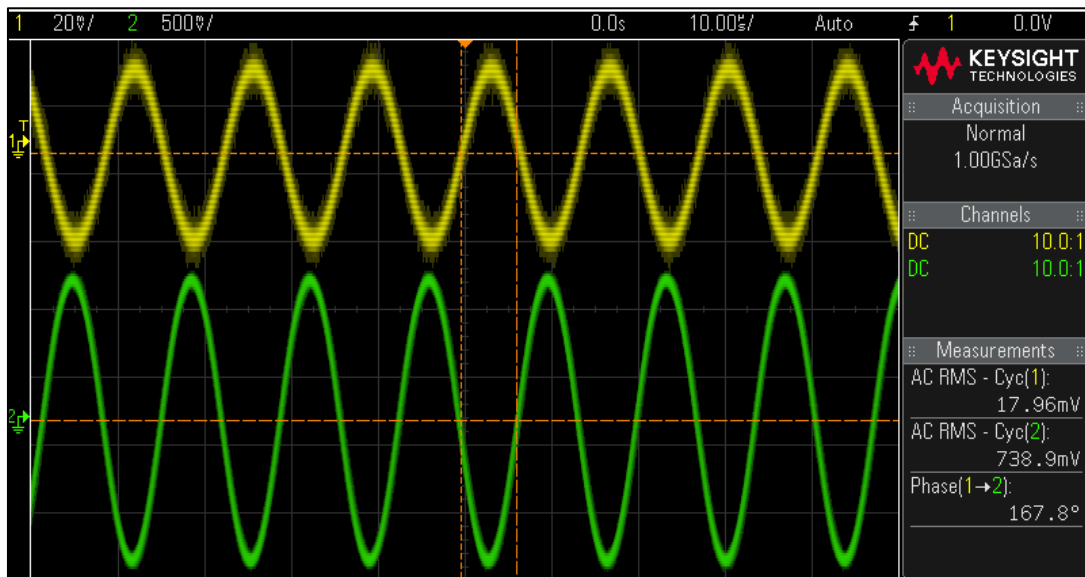
Figure 4: Actual First Stage response to a 25mVpp 71kHz Sine Wave
