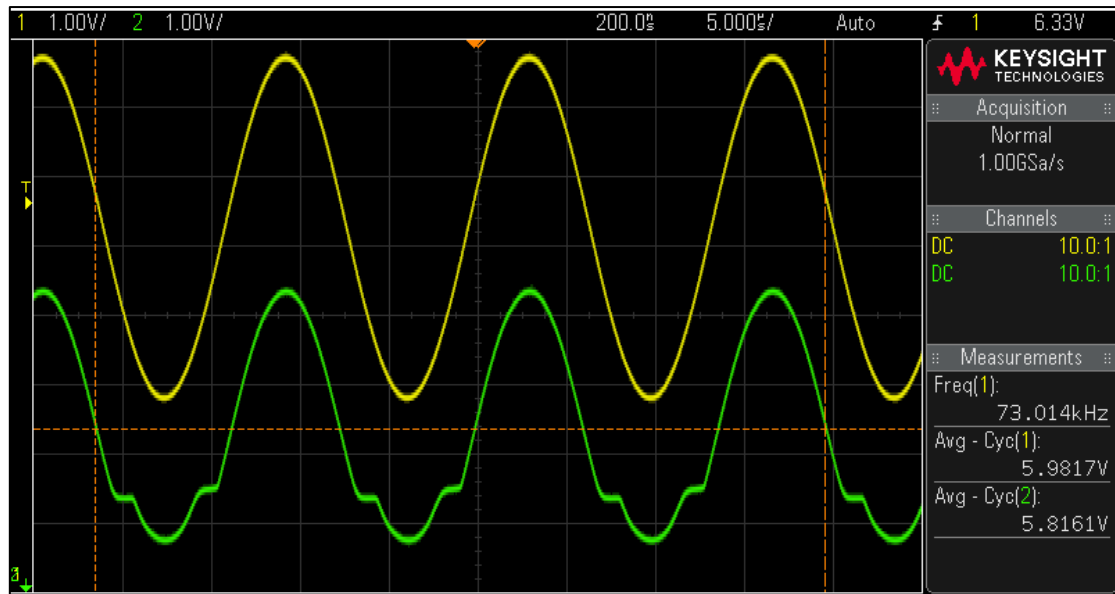
Figure 10: Actual Third Stage Response to 25mVpp 71kHz Sine Wave
